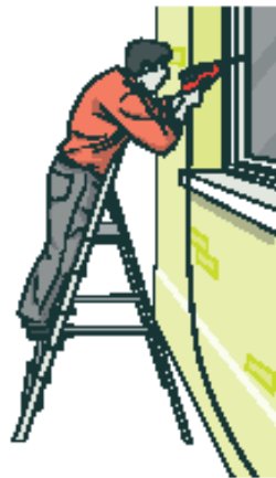
CORRECT ✓ Steps facing work activity
